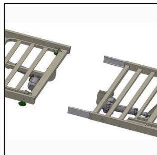
Figure 8: Connecting platform sections
